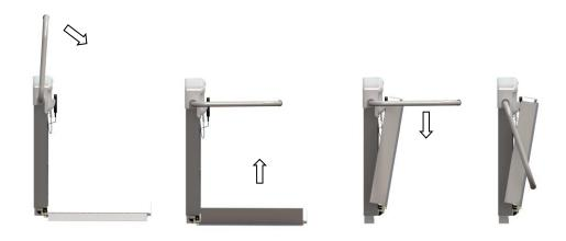
In order to unfold the platform again, one should proceed in reverse order and in conclusion fold up the safety gate of the desired access point to a completely upright (vertical) position.
