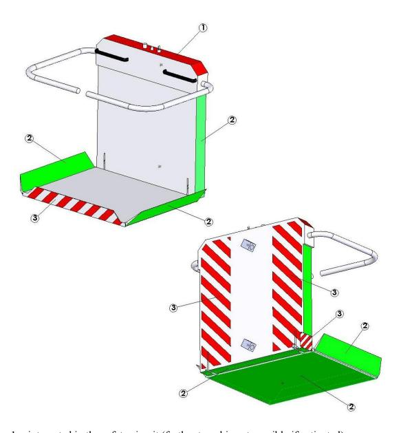
1 = integrated in the safety circuit (further travel is not possible if activated)
