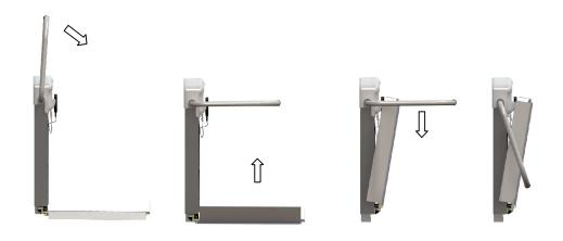
Proceed in the reverse order to open the platform again and finally raise the safety barrier at the desired access point right up to the top (vertical).
