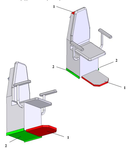
1 = integrated in the safety circuit (further travel is not possible if activated)
